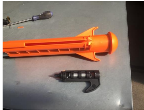
3. Remove the black plastic hook-system incl. inside parts
