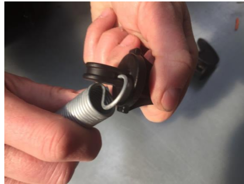
5. Assemble the spring and the black plastic cap
