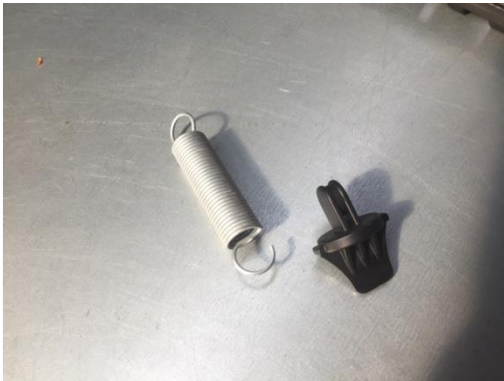
3. Remove the black plastic hook-system incl. inside parts
