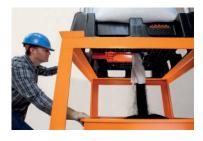
Bottom discharge with dosage and cut off possibility through the slide of the Indus Neva System
