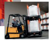
Movement of Indus Neva Systems by a forklift truck (max.  $2 \times 1.500$  kg.)
